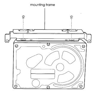
3. Repeat step 2 to attach a mounting frame to the other side of the drive.
